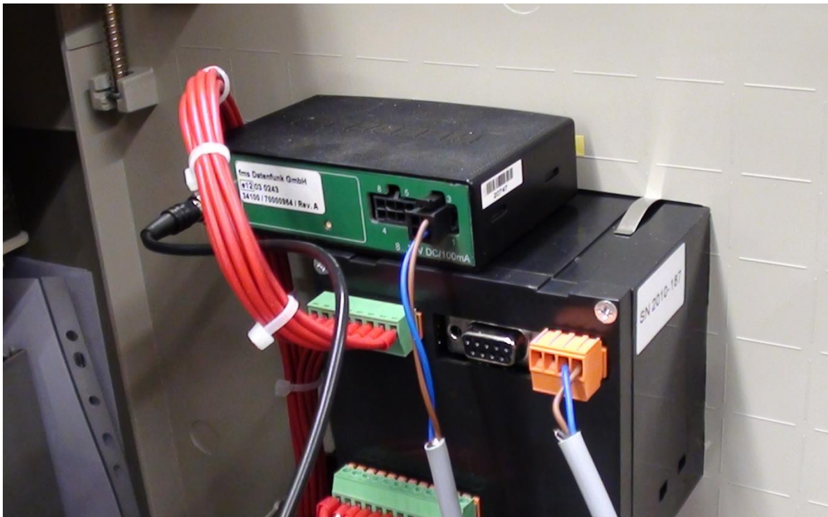
Fig. 2.1: Connection of GPS module with Pro module
