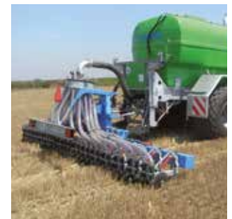
Slurry injector Innovative spreading technology
