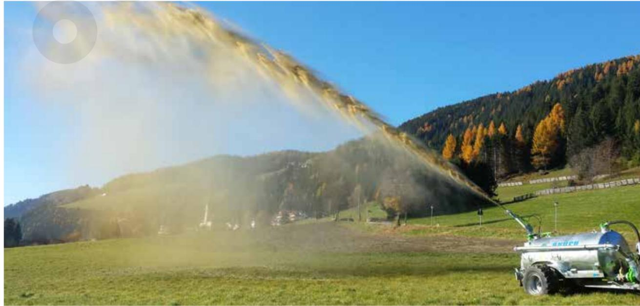
**Proven vacuum technology paired with high spreading pressure**
