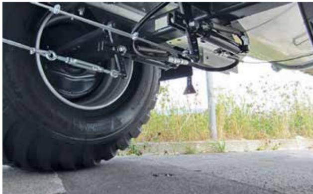
**Pressure limiting valve for hydraulic braking systems**
