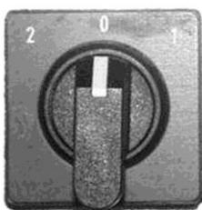
3. Align the towers flush with the centre tower by using the tower alignment switch (*take aim on drive motors*).
