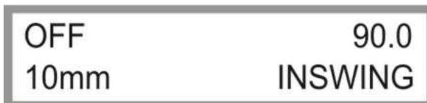
Adjust this angle by loosening the driver screw of the encoder in the collector and by turning it until 90° are displayed on the control panel. You may also correct the angle in the machine parameter menu on the control panel. See in this context the operating instructions of the control unit *Centerliner Standard PRO* under separate cover.
