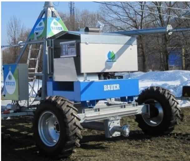
The Diesel generator unit supplies directly the control centre of the CENTERLINER.
