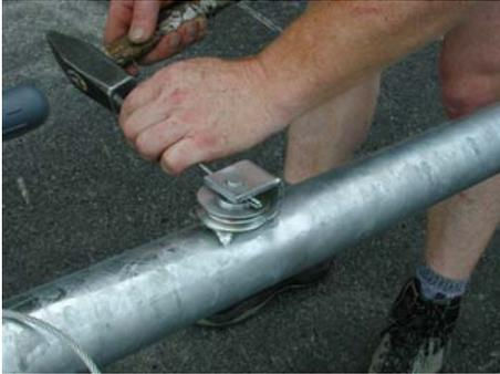
Remove the deviating roller from the mixer shaft...
