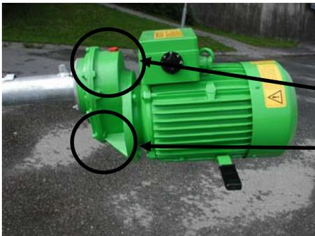
The gearbox of the **MEX 450 G** is filled with **0,3 l** oil type Shell X15W/40. Here, too, the oil only needs to be exchanged in the course of repairs.
