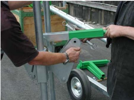
Lock the adjusting spindle in the mixer shaft support.
