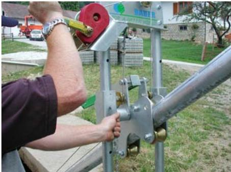
Before you put the mixer into operation, make sure, that the mixer shaft as well as the roller carrier are secured with the corresponding safety pin.
