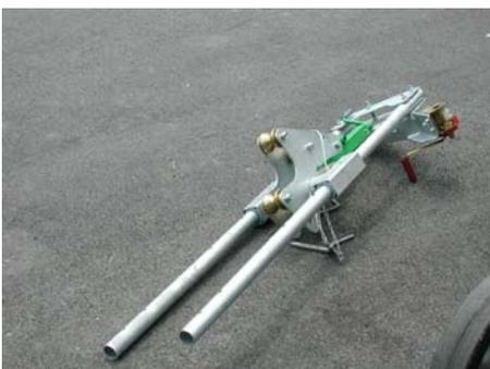
Then screw the guiding pipe with the mixer shaft support and the rope winch to the two-wheel frame.
