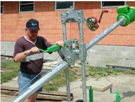
Crank up both supports until the wheels are definitely off the ground. If you have a concrete ground, we recommend to cut in slits for the supports. These supports together with the front support plates absorb the pushing forces occurring during the operation.
