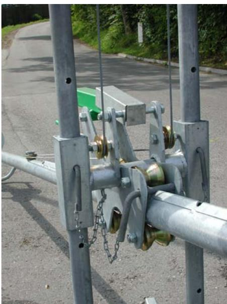
The rollers of the mixer shaft support, the guiding pipe, the bearing of the tires as well as the spindles of the support, have to be lubricated, as required, with a tenacious grease that adheres well.
