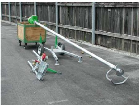
Place the mixer shaft onto the two-wheel frame and support the motor.
