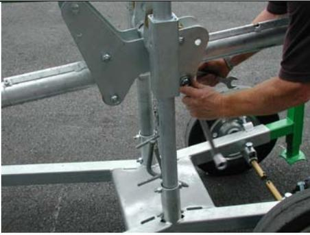
... put the mixer shaft support on the mixer shaft and
