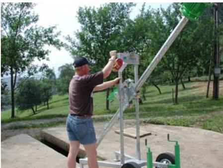
If your pit has a small opening, the mixer shaft support must be fixed in the upper rest position at the guiding pipe with the rope winch and the mixer shaft tilted strongly with the hand lever spindle
