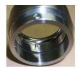
When mounting the rotating collar ensure that bolt and groove are properly aligned (misalignment will bend the pin when force is applied and the spring is pressed away ensuing excessive pretension of the sliding faces).
