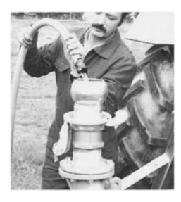
Fill up pump and suction line completely with water through the delivery socket.
