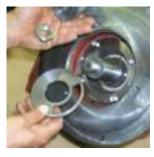
Assembly kit for adjustment of the functional length of the mechanical seal.
