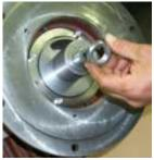
it the space-adjusting nut - mounting length  $47.5 \pm 0.5$ mm.
