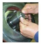
Press on the mechanical seal with the help of the sleeve (remove the sleeve again).
