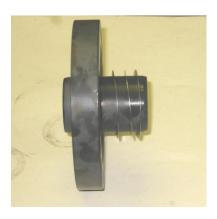
6) Install the mechanical seal, the key and the hub with right number of shims on the pump shaft and fasten again the hub with torque of 250 Nm.
