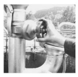
• Couple the delivery line and close the stop valve in the delivery line.
