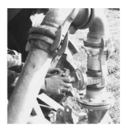
Connect the delivery line and close the stop valve in the delivery line.
