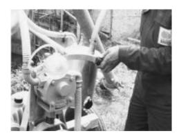
Shift lever to position 2 (lift up) and hold it until the pump is filled.
