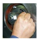
Use Allen key to tighten (fix) the threaded bolts that have been moistened with Loctite.
