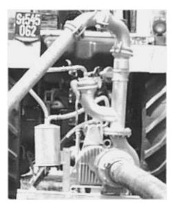
Make connection between side branch and tank (quick coupling).
