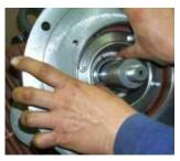
**Mount the stationary seal ring**Groove and anti-rotation lock pin must be in alignment.
