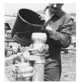
• Always fill up the pump with about 3 litres of water through the side branch of the delivery socket.
