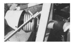
Connect tractor and pump by means of the drive shaft.
