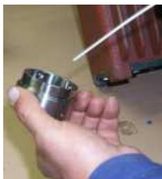
Spray the O-ring with lubricant inside
