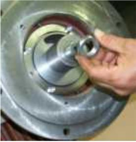
it the space-adjusting nut - mounting length  $47,5 \pm 0.5\text{mm}$ .
