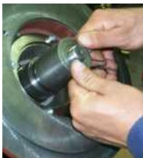
Press on the mechanical seal with the help of the sleeve (remove the sleeve again).
