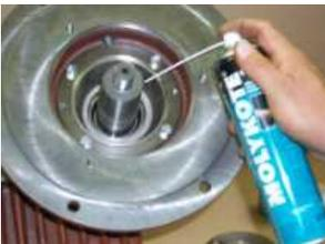
**Spray the O-rings with Molykote to reduce friction.**
