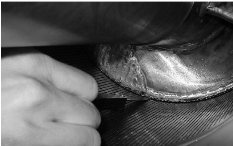
Fig. 13-15 Measuring of the working gap between the screen and the auger; the gap is measured on the bottom side of the screen while the machine is at rest. The measurement yields two times the working width because the screen rests on the top of the auger when the machine is not running.
