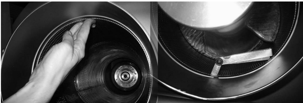
Fig. 13-11 Movable screen in the separator, inspection of the floating capacity by hand (left)
