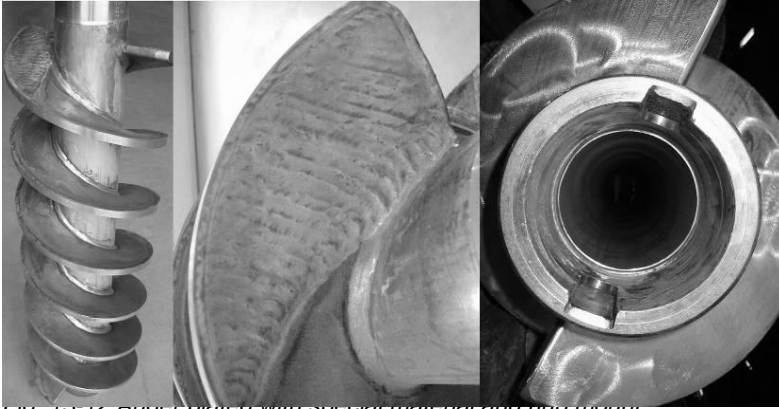
Fig. 13-12 Auger plated with special material and hub mount, new condition
