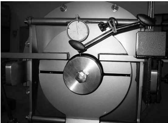
Fig. 13-13 Inspection of the auger axial eccentricity
