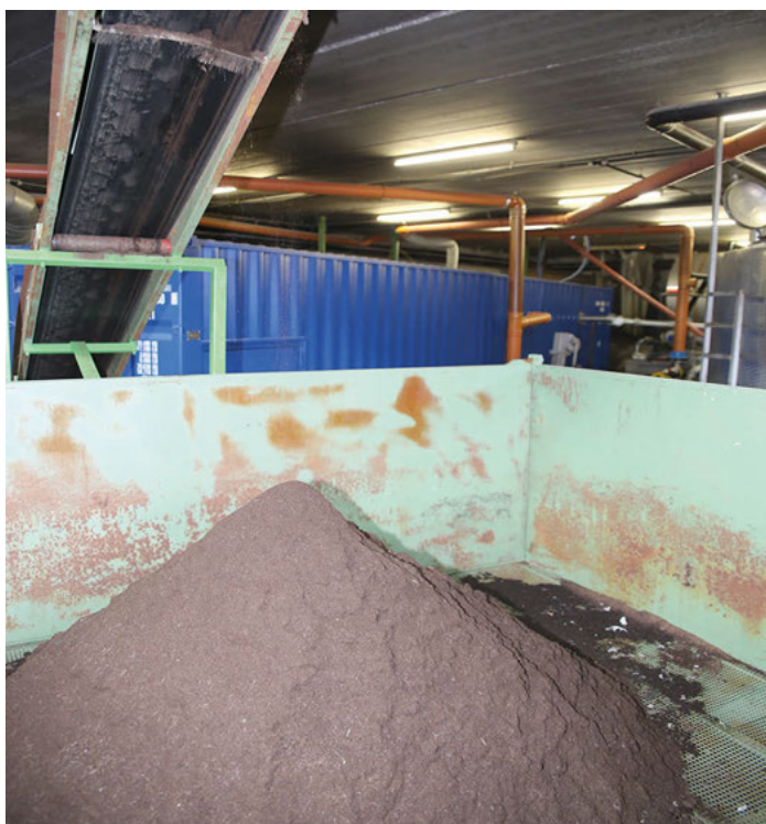
After leaving the drying drum the bedding material is dry and clean, and will store for up to a week under cover. Liquid is pumped away to a slurry lagoon before being applied to the land.
