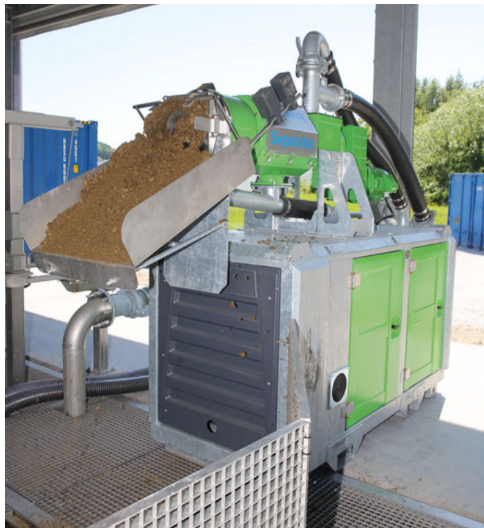
The new mobile separator from Bauer is designed to be easily moved between sites. It is available as a standard separator or as a green bedding separator producing green bedding material at a dry matter content up to 36 per cent and with a work-rate of 25m 3 /hr.
