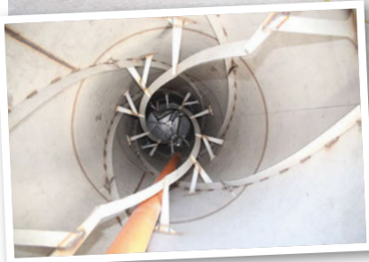
The larger BRU1000 and 2000 bedding recovery units are suitable for herds up to 2,000 cows and consist of a green bedding separator installed in a 20ft container mounted above, and feeding into, the revolving drum which is in a second 40ft container. The two containers make up one BRU system, awaiting dispatch from Bauer's factory. (pictured left), the inside of the drum.
