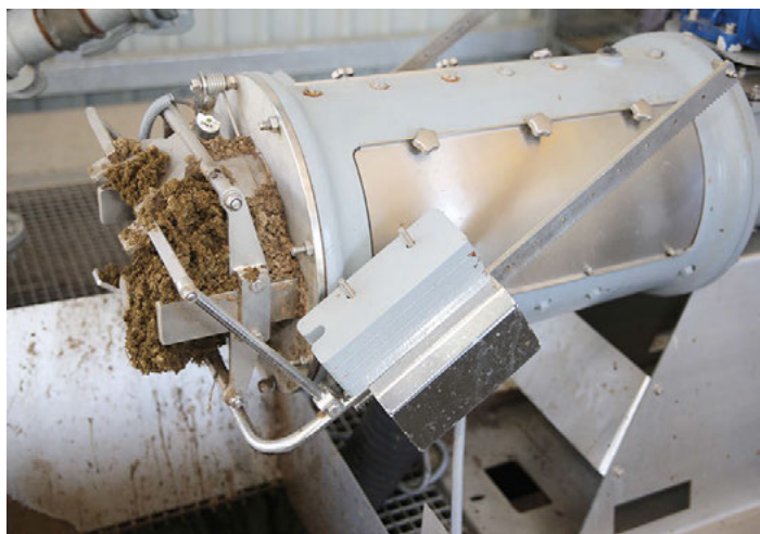
FAN Separator green bedding separators are available with additional features over Bauer-branded units. Constant feed can be maintained with a built-in agitator at the slurry entry point and automatic adjustment of the plug pressure can be achieved by the optional automatic weight adjustment which alters the position of the resistor weights during operation.
