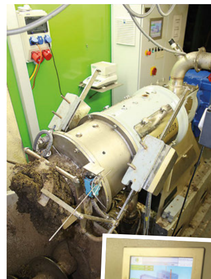
The BRU Compact bedding recovery unit installed on a farm near Voitsberg, Austria. The new Compact version is designed for smaller herds of approximately 600 cows and produces dry green bedding up to 46 per cent dry matter. In one end of the container is the green bedding separator (pictured), and from this the green bedding enters the 6m drying drum in which it achieves a temperature of 65°C during the aerobic reaction.
