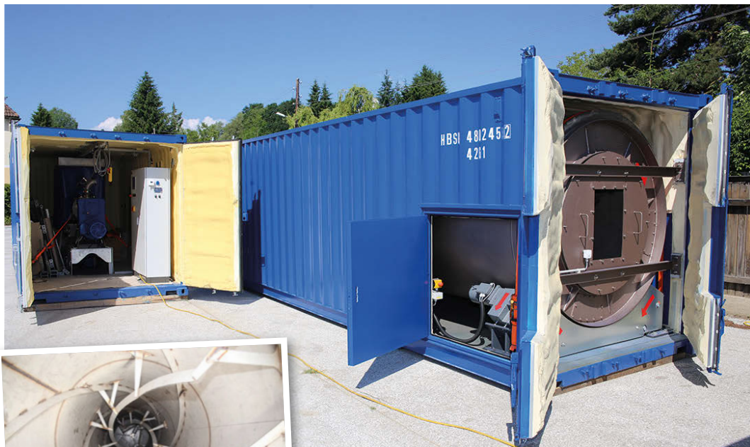
The larger BRU1000 and 2000 bedding recovery units are suitable for herds up to 2,000 cows and consist of a green bedding separator installed in a 20ft container mounted above, and feeding into, the revolving drum which is in a second 40ft container. The two containers make up one BRU system, awaiting dispatch from Bauer's factory. (pictured left), the inside of the drum.
