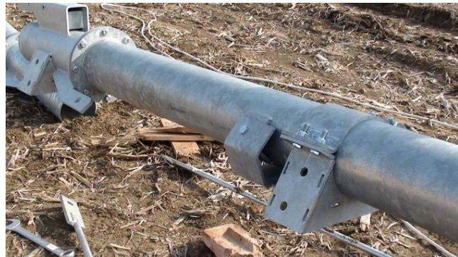
Installation of the bracket and clamp for fastening the drive tower legs to the main pipe
